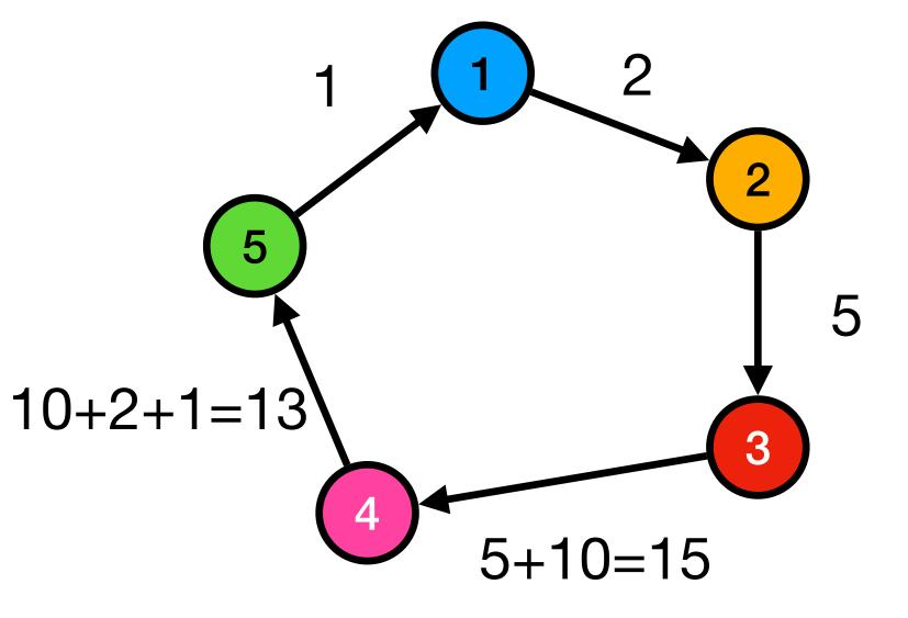
Worse algorithm: charge the weight of the path from each non-sampled vertex to its nearest sampled vertex in the contracted Euler tour
